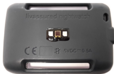
Back of arm module: with CE and WEEE symbol
