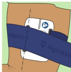
Use the remaining end of the elastic strap to measure the circumference of the wearer's arm above the biceps in a bent position. Do not stretch the strap.
