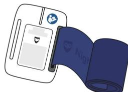
The elastic strap should be adjusted to the size of the upper arm of the wearer. One side of the elastic strap has already been fitted into the sensor.
