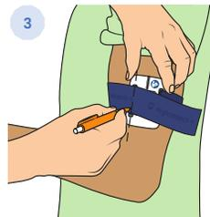
Mark the elastic strap where it overlaps the second sensor clip entrance and cut the elastic strap at the marked point.
