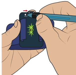
If you wish to turn the sensor OFF to prevent the battery from running out, use the ON/OFF switch to turn the sensor OFF. The sensor cannot charge when it is switched OFF.
