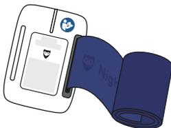
The elastic strap should be adjusted to the size of the upper arm of the wearer. One side of the elastic strap has already been fitted into the sensor.
