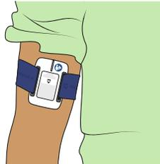
**PLEASE NOTE:** In order to achieve as accurate detection as possible of any epileptic seizures, the sensor should be worn on the upper arm (biceps) and directly on the skin. If the wearer is wearing a pajama top or other long-sleeved garment, please ensure the sleeve is wide enough to wear the sensor underneath or else seizure detection is not possible.
