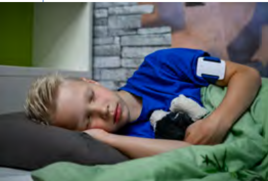
Wearable sensor that detects seizures using Photoplethysmography (PPG) and Accelerometry (ACC) sensors
